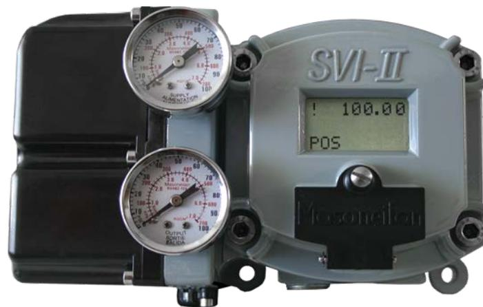
BHGE's SVI II AP positioner with proven electronic and pneumatic technologies, combined with multiple sensors and smart software, offers high performance valve control with real-time diagnostics. The SVI II AP positioner is configured with a non-contact position sensor, a 32 bit ARM processor, a rugged I/P, and a poppet valve volume amplifier.
