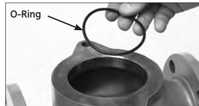
Figure 7a - Remove cage, seat, and o-ring
