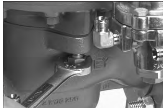
Figure 27 - Tightening the body cap screws
