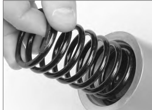
Figure 18 - Removing the main spring
