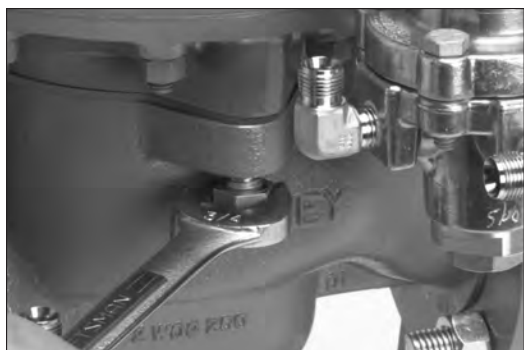
Figure 43 - Tightening the body cap screws
