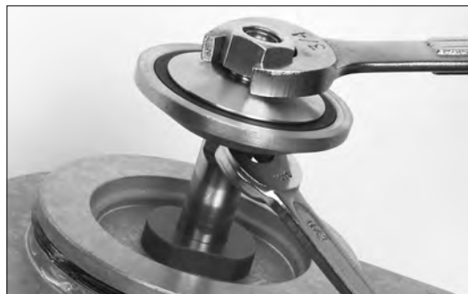
Figure 51 - Remove the stem nut
