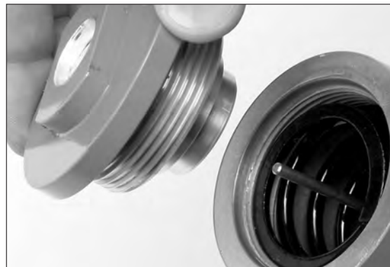
Figure 48 - Installing the spring case cap
