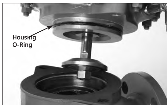
Figure 42 - Installing the actuator on the body
