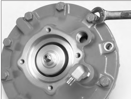
Figure 29 - Removing the housing cap screws
