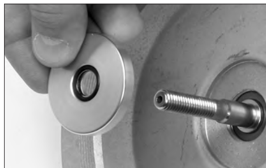
Figure 32 - Installing lower diaphragm retainer
