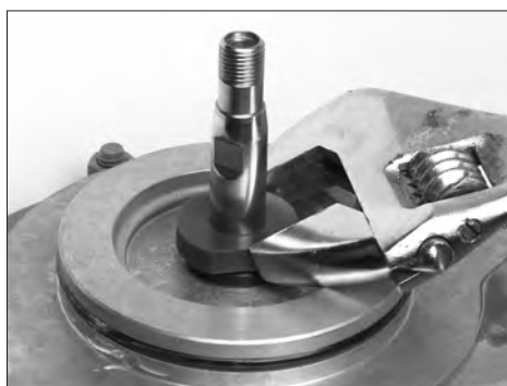
Figure 10 - Removing the stem bushing
