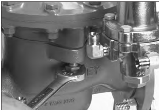
Figure 17 - Tightening the body cap screws
