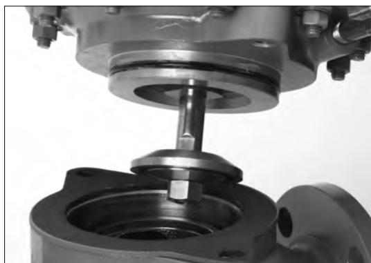
Figure 50 - Remove the actuator housing assembly
