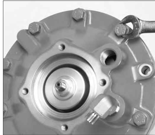
Figure 35 - Install the remaining actuator cap screws
