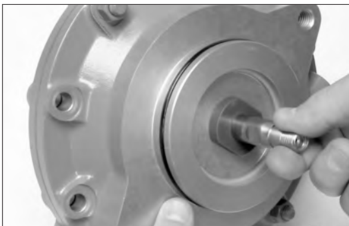
Figure 34 - Checking stem for free movement
