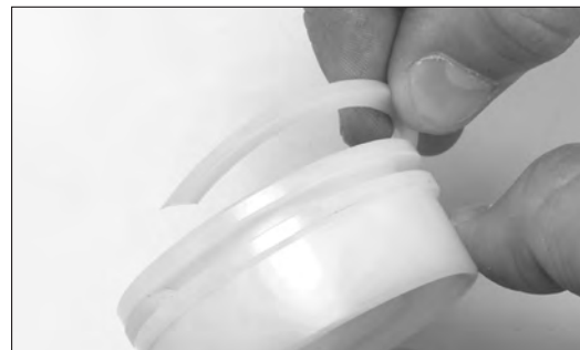
Figure 37 - Installing piston ring on piston
