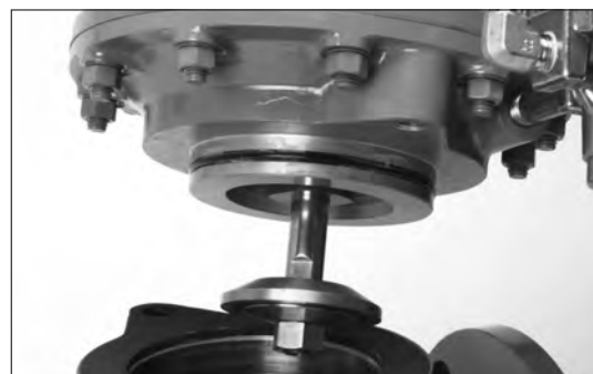
Figure 28 - Removing the main actuator
