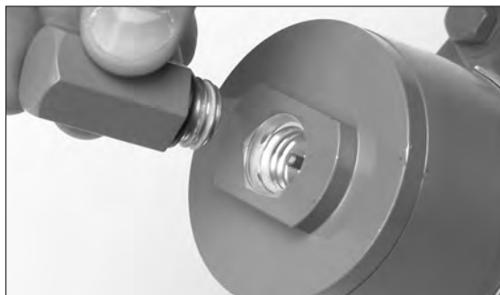
Figure 49 - Installing the indicator cover
