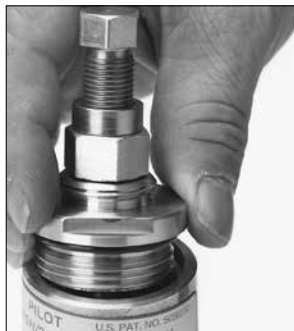
Figure 23 Installing the closing cap assembly with spacer (to prevent spring over compression) for Pilots with the Black and Green Springs.
