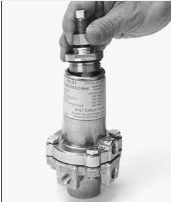
Figure 22 Installing the closing cap assembly for Pilot with the Red, Plated, Blue, and Purple Springs.
