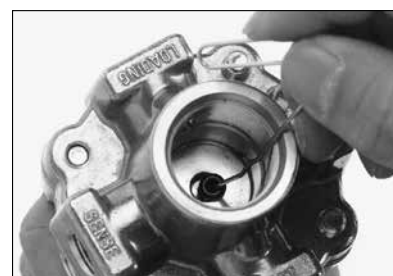
Figure 16 A paper clip easily extracts the O-Ring out of the pilot body.
